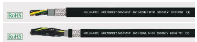
MULTISPEED® 500-C-PVC high flexible, safety against high bending in drag chain systems, oil resistant, low torsion, screened, EMC-preferred type, meter marking
