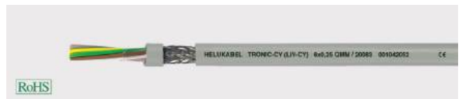
TRONIC-CY (LiY-CY) flexible, Cu-screened, colour coded to DIN 47100, EMC-preferred type, meter marking
