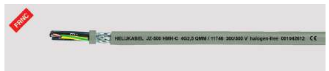
JZ-500 HMH-C flexible control cable, halogen-free, extremely fire resistant, oil resistant, Cu-screened, EMC-preferred type, meter marking
